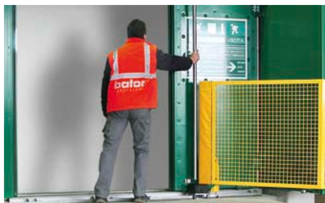
Fully assembled cross passage door in the opened state. Collano adhesives are a key element of these safety doors being installed in what will once be the world's longest railway tunnel (57 kilometers).
