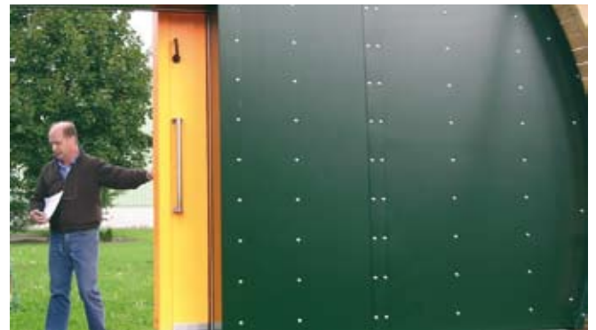
Sliding firestop door for the Sierra Guadarrama high-speed rail tunnel in Spain. Nikolaus Schindler, responsible for development & engineering at Hodapp, shows the prototype: «We obtained the best test results with systems bonded with Collano».
